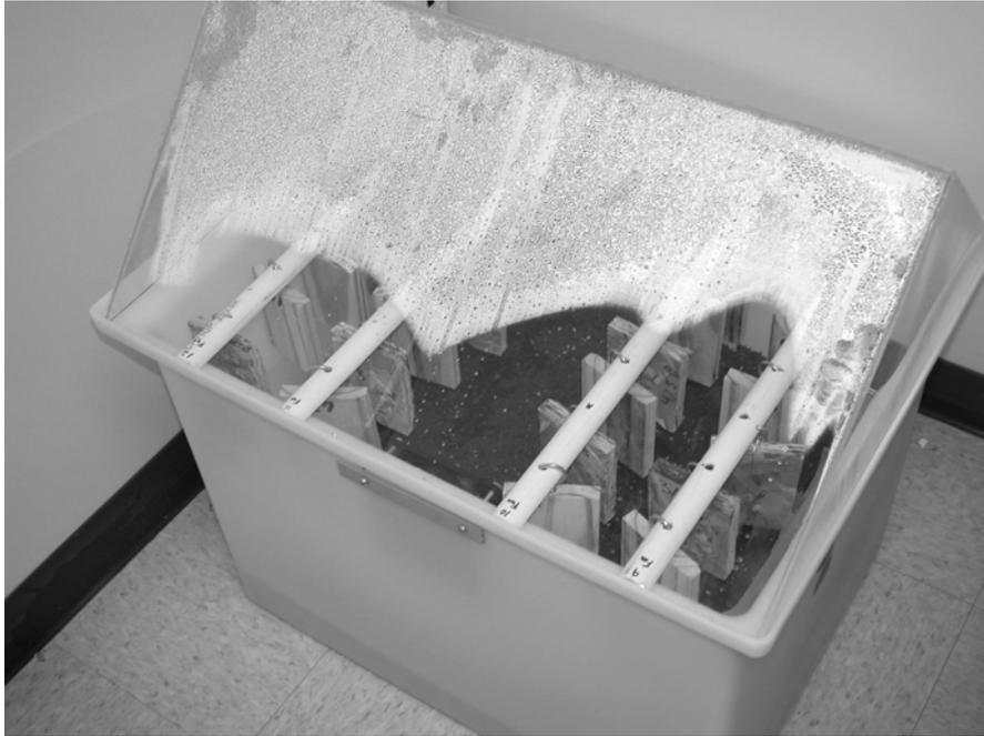
Figure 3: Environmental chamber for testing wood-based products for resistance to mould.
