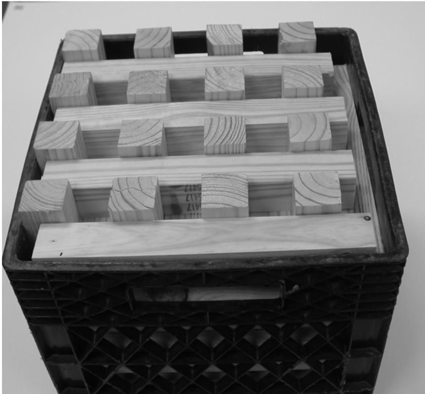
*Figure 2: Bait crate for collecting termites or testing products.*
