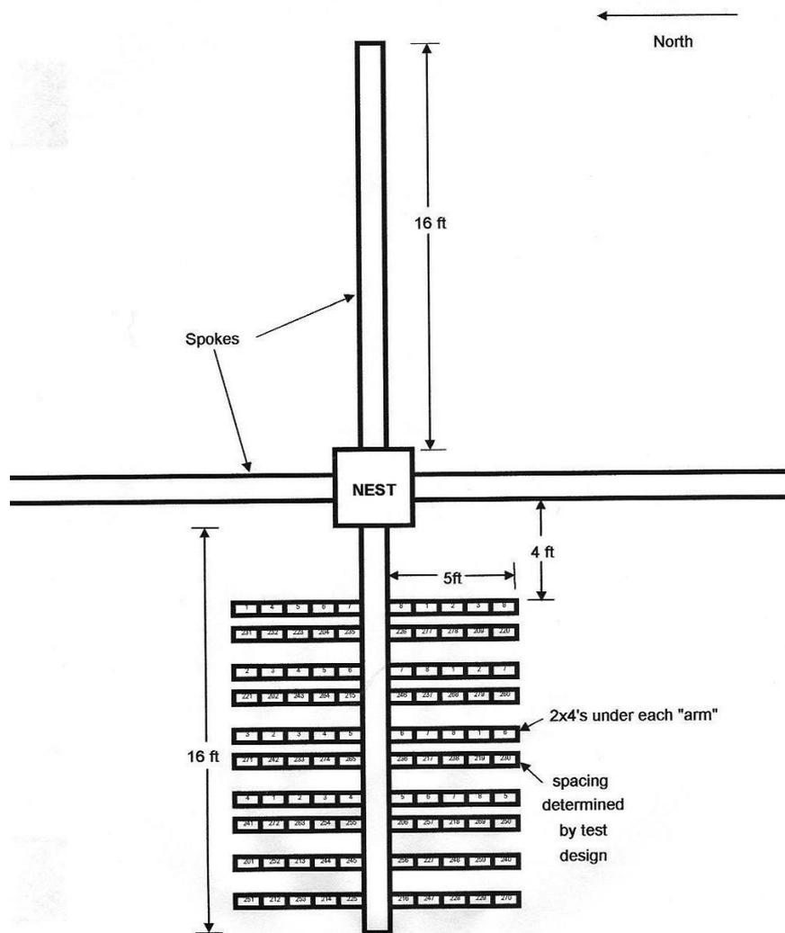
Figure 1: Schematic of enhanced termite field site.
